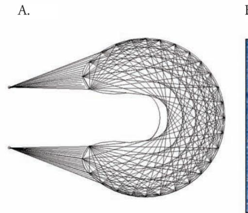
**FIGURE A.** THIS UNIQUE FIBER NETWORK DESIGN ENABLES THE SCAFFOLD TO SUPPORT MECHANICAL LOADS IN THE KNEE.
